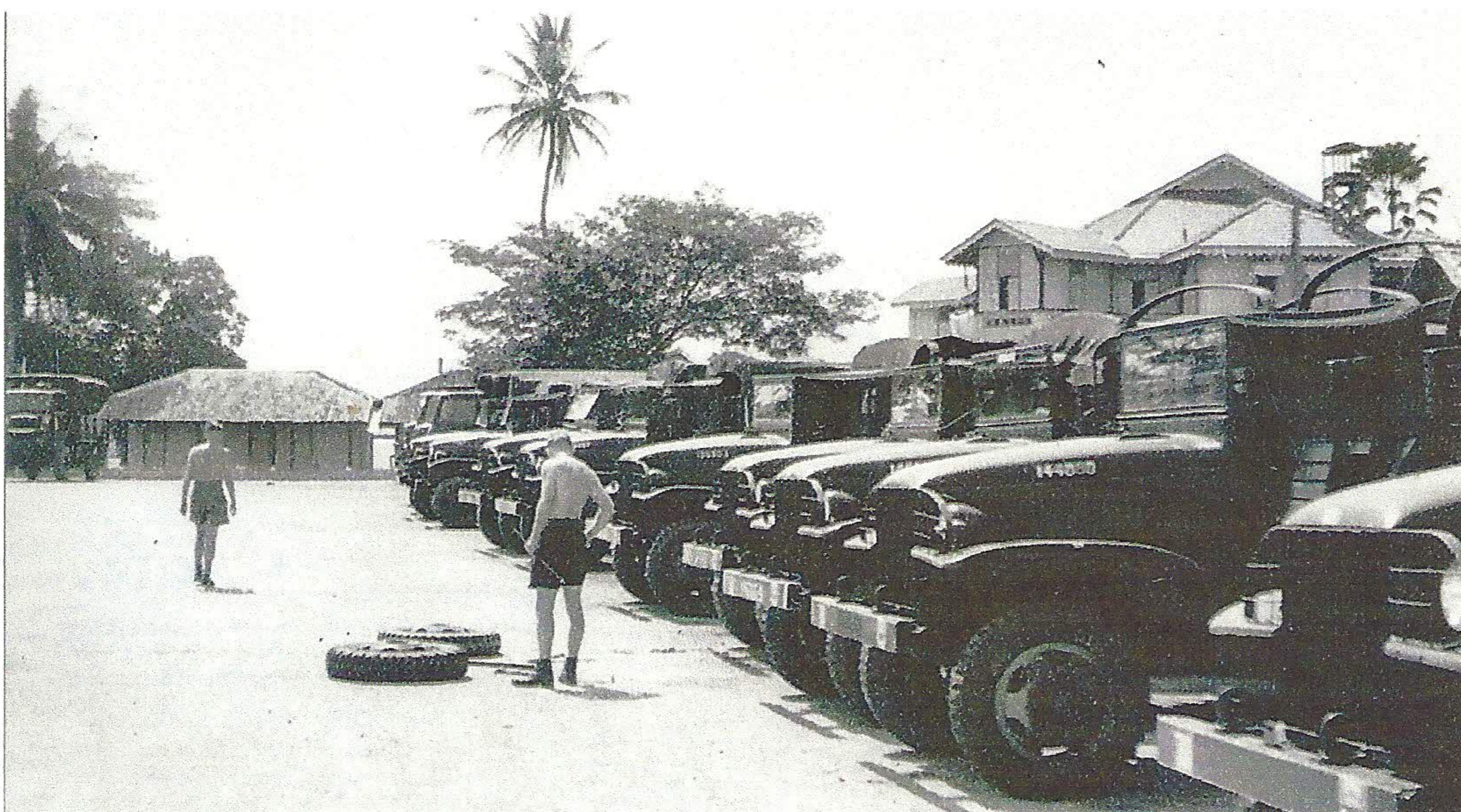
Running Repairs - Tyres had a 10 month life span.
